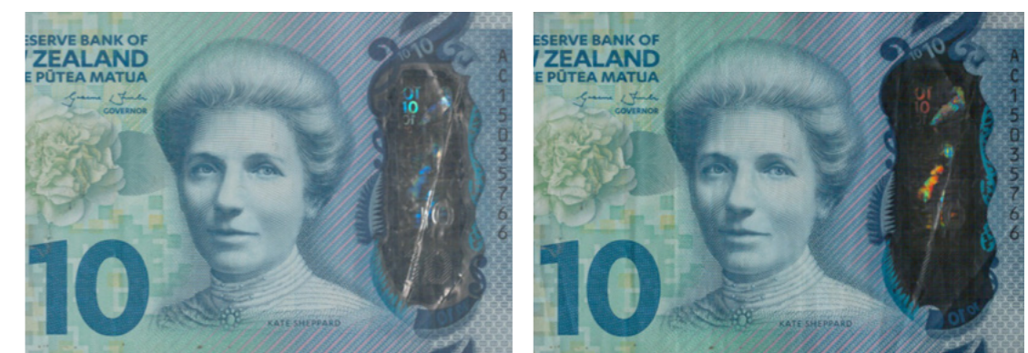
FIG. 5 - BALANCED AND ASYMMETRIC ILLUMINATION IMAGE VIEWS HIGHLIGHTING THE DEGRADATION IN THE OPTICAL ACTIVITY OF THE HOLOGRAPHIC FOIL
