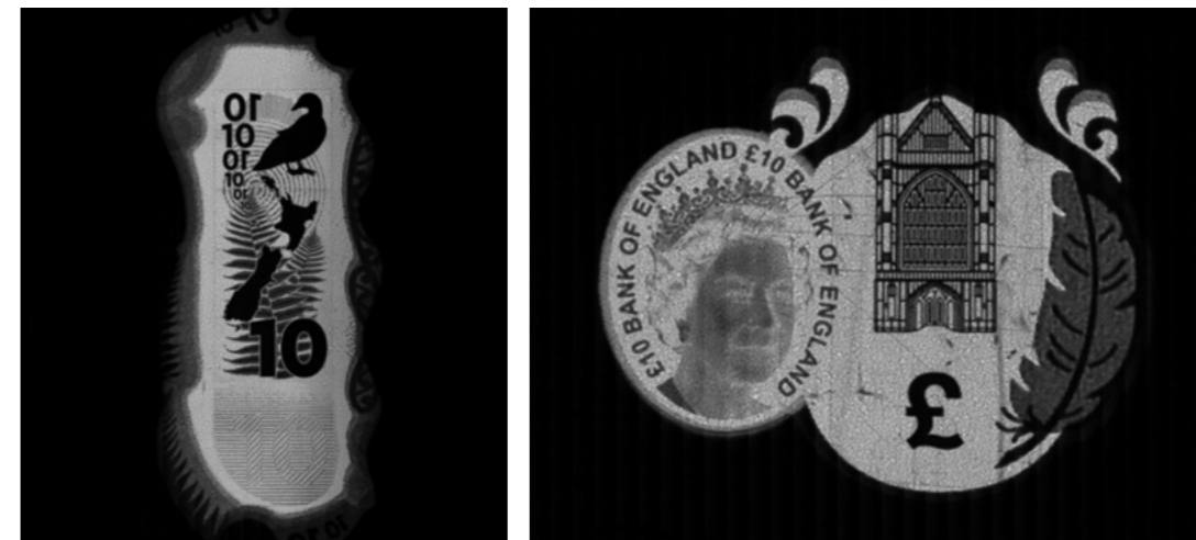
FIG. 8 - IMAGE SEGMENTS OF HOLOGRAPHIC FOILS AS SEEN BY THE SHADOW MASK TRANSMISSION VIEW OF GEMVISION
