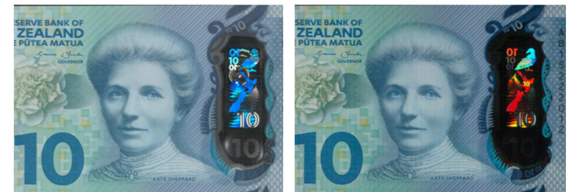
FIG. 4 - CHANGE IN APPEARANCE OF THE HOLOGRAPHIC THREAD UNDER TWO DIFFERENT ILLUMINATION CONDITIONS
